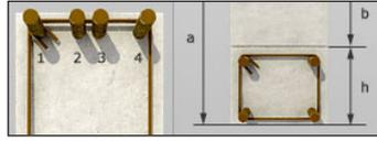
Inserting the binding joist with the insertion of longitudinal reinforcement and stirrups.
