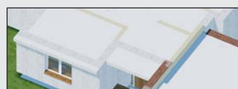
Inserting automatic ceilings on the closed external walls contour.
